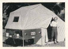
minute. For off-season use, removal of camp unit converts Heilite into rugged utility carrier. Trailer light weight at 310 lbs., with low silhouette. Individually-suspended and cushioned wheels, connected by "no-sway" torsion bar.
