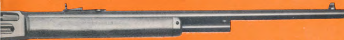
Marlins Model 1895 differs in appearance from their original model. The new model has a round breechblock instead of a square one. Marlin advises that loads should not exceed those recommended by the factory.
