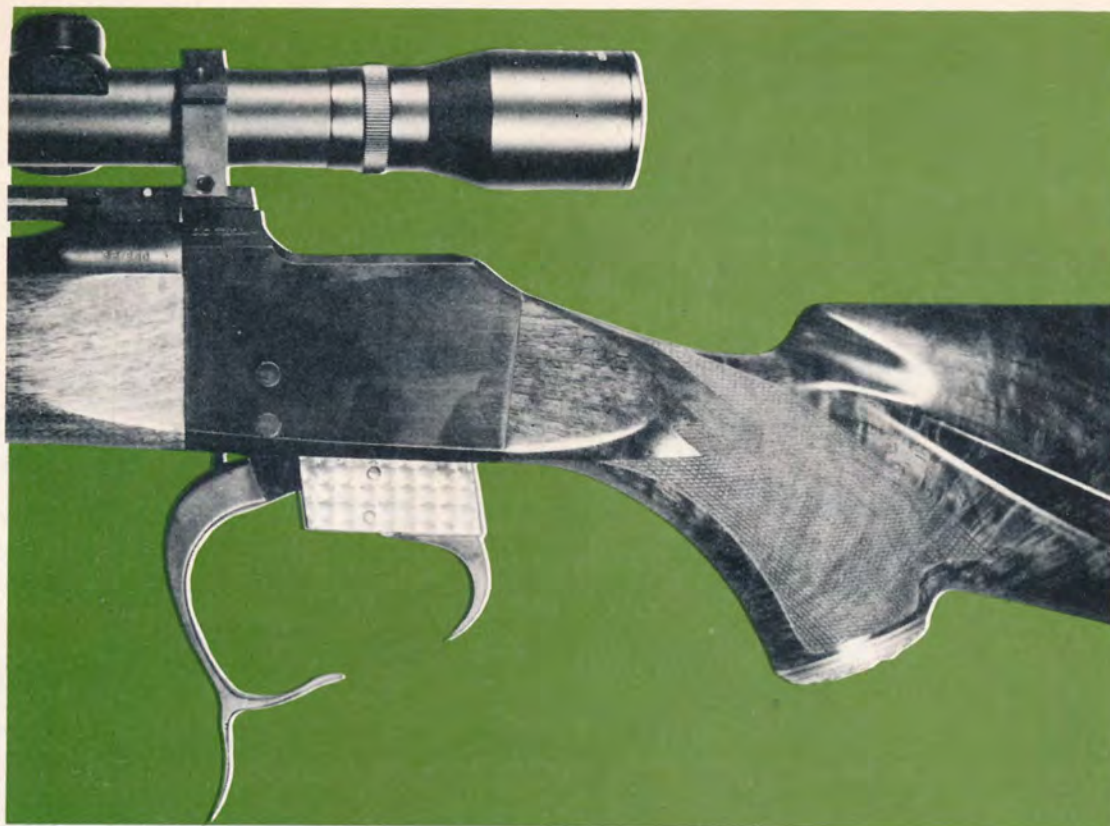
This close-up shot illustrates how the finger lever, when moved downward and forward, acts to depress the spring-loaded extractor.
