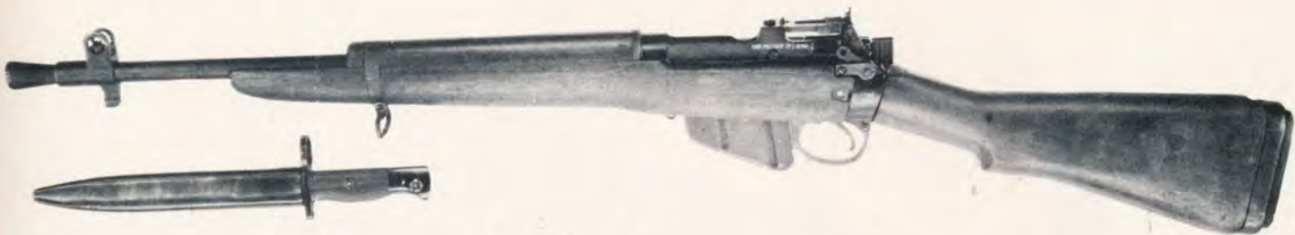
The No. 5 Lee-Enfield, which was specially designed for jungle fighting. The rifle proved to be a most effective weapon in that role. Note the attached flash eliminator. The No. 5 was the only Enfield to be fitted with such a device.
