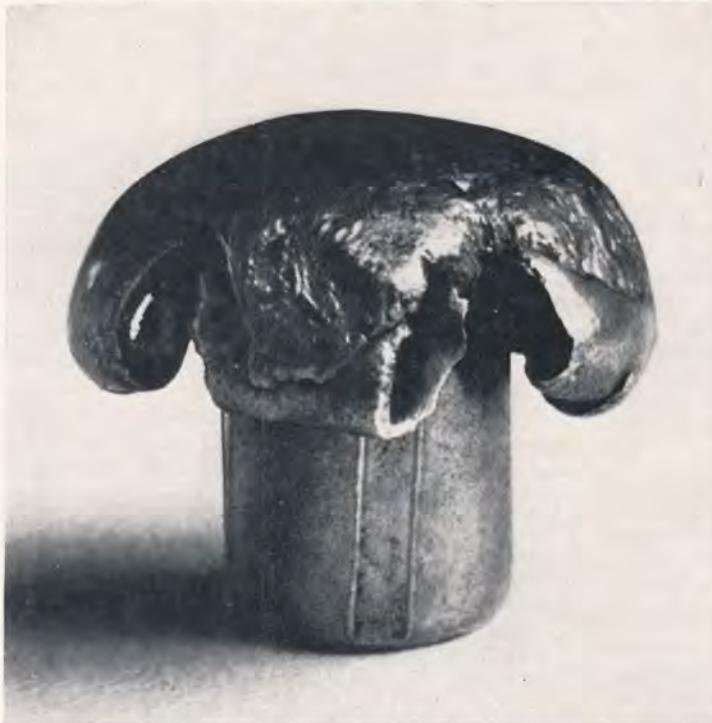
This "Core-Lokt" bullet still retained 62% of its original weight when recovered from a Kodiak bear.
