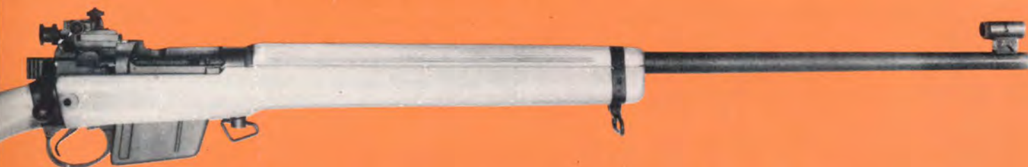
The latest version of the Enfield, which has been dubbed the "Enfield Envoy." The rifle embodies the No. 4 Rifle action, The No. 8 Rifle woodwork and has been fitted with the Enfield heavy "Target" barrel and equipped with Match sights.
