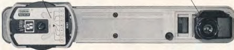
Interchangeable scale (scale shown #8). Example: Scale #8 for 30-06, 180 grain bullet. Rifle zeroed at 200 yards. Holdover at 300 yards—9 inches.
