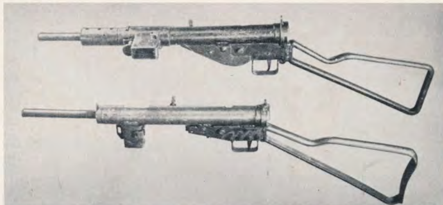
The Sten Mark II (top) and the German imitation known as the MP 3008. Germany manufactured several imitation models of the Sten in WWII.
