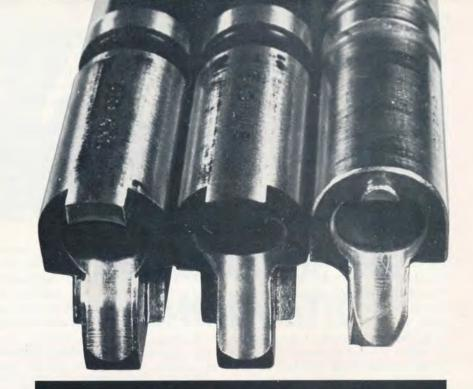
The Browning chamber illustrated on the right clearly shows the smoothly radiused mouth which will prevent case-mouth snagging. The center barrel has a small amount of radius, but the left barrel has none and causes jams. The left barrel also shows the new straight Smith and Wesson M39 ramp as it is compared to the hump-shaped ramp of older M39s.
