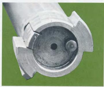
The bolt face on the HVA-Gustaf action is unique only in that it utilizes dovetail locking lugs which greatly add to the smoothness of operation and virtually eliminates any trace of bolt wobble for added glidability.
