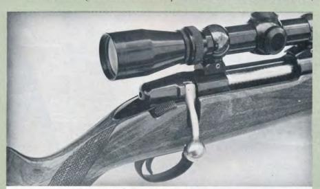
The bolt handle on the new HVA action fits into the receiver slot, where it acts as a third lug. The safety was positive and quiet.
