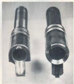
Browning HP full length ramp barrel on left handle the high performance loads best, while segmented Colt ramp, right, requires more fitting.
