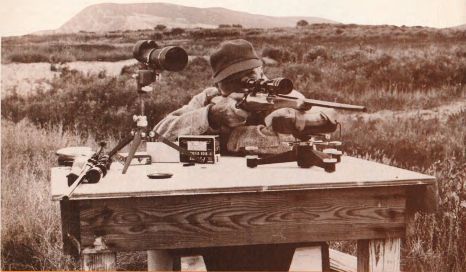
A rigid shooting bench and the use of a sand bag rest are of tremendous aid to the hunter when trying to sight in his rifle. Aiming error can be reduced dramatically if the scope has been mounted properly.
