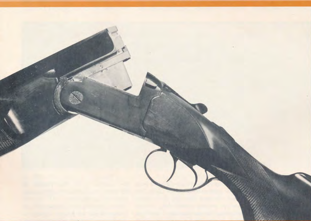
Pictured is an action-open view of the M-810, showing its locking lugs in profile and its stirrup-type extractor. The barrels are of Boehler steel and the chambers are cut with extra long forcing cones to reduce pellet deformation.
