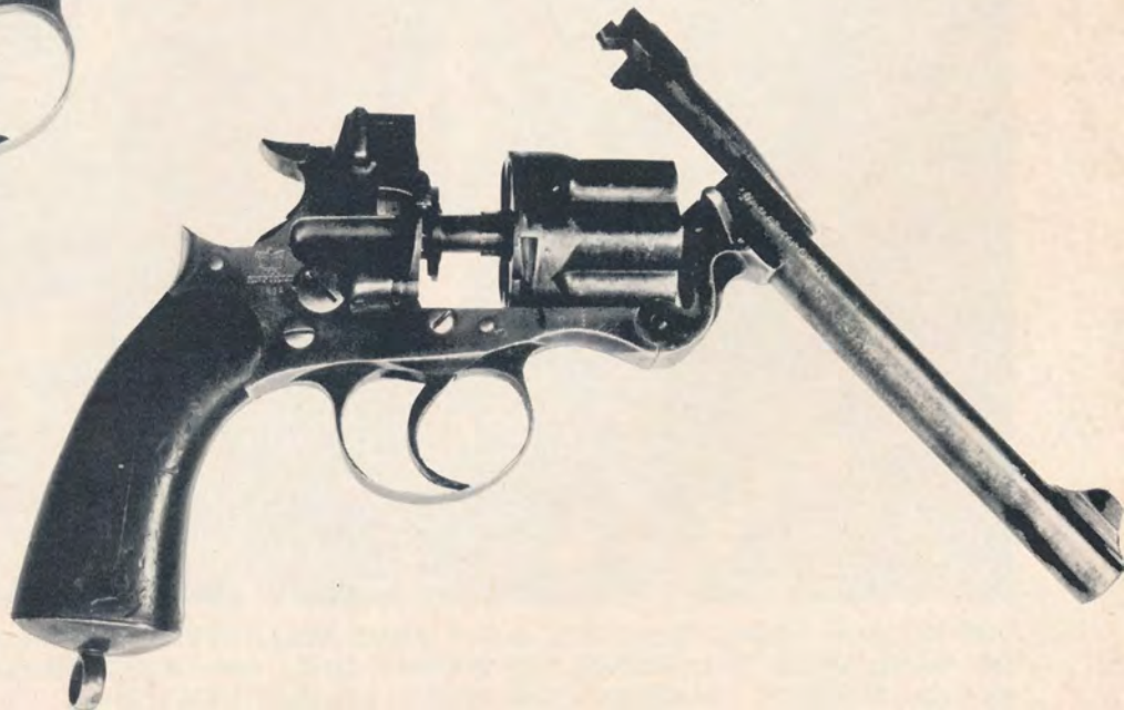
The Enfield .476 revolvers took the place of the Adams in the British forces between 1880 and 1887. Its rapid ejection system differs greatly from that of the earlier Smith & Wesson. The top-break, hinged-frame weapon was made to fire the new .476 round.
