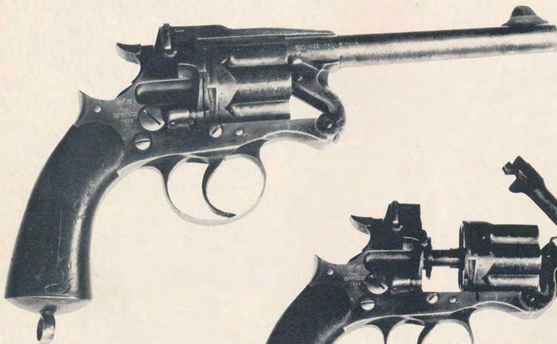
The Enfield .476 revolvers took the place of the Adams in the British forces between 1880 and 1887. Its rapid ejection system differs greatly from that of the earlier Smith & Wesson. The top-break, hinged-frame weapon was made to fire the new .476 round.
