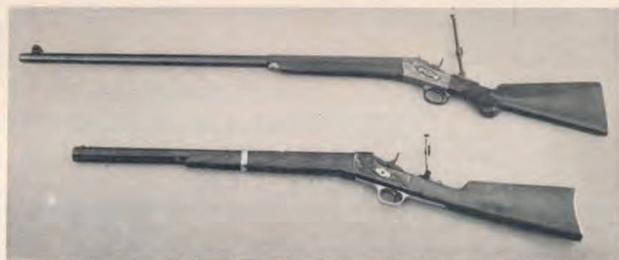
This photo shows the Navy Arms Rolling-Block rifle (lower) beside an original Remington Rolling-Block Creedmoor and graphically illustrates the points made in the text concerning the short, un-tapered barrel, the barrel band, hammer spur and trigger shape, along with the brass guard of the Navy Arms Rifle.
