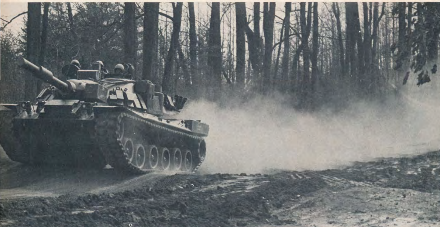
A prototype of the Army's Main Battle Tank for the 1970s (MBT-70) traverses a cross-country course at Aberdeen. The author states that Germany produced the best tanks during the war and now Russia is doing so.
