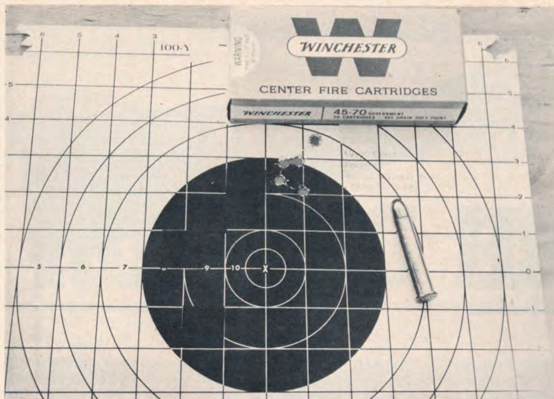
One of the better targets fired with the Navy Arms Rolling-Block rifle. This 1½ inch group at 100 yards was made with handloads comprising 350-grain Herters round-nosed soft point bullets and 56-grains H-4831, with CCI #250 Magnum primers. The cases used were the modern solid-head Winchester-Westerns, composed of a fine, strong brass. The Winchester-Western ammo was the most accurate factory round tested.
