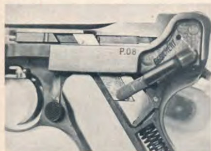
The Luger's sear pivots laterally; the safety blocks it so it can't swing out and release the striker.
