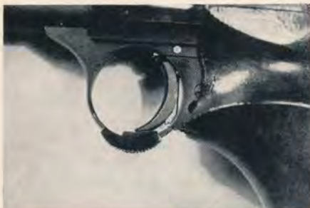
This elementary safety is a sliding wedge on the trigger guard, which blocks the trigger like a door jamb.
