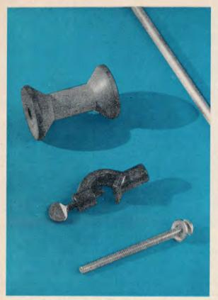
Necessary for the rest are thumb screw, 36" rod, wood spool and a thru-bolt.
