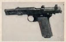
The slide on this 1911 Steyr is presently being held open for loading by the thumb safety. Note the lever centered above the grip panel which both releases the cartridge column for unloading and depresses the follower so that the slide may be run forward.
