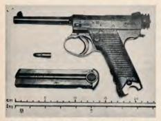
The bolt on the Pattern 14 (1925) "Nambu" is held rearward on the last shot only by the magazine follower, and slams shut when the magazine is removed. Photo, courtesy of M. H. Josserand.
