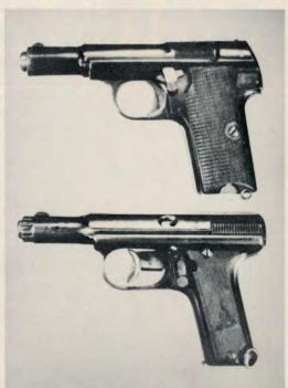
Ecia shows a strikingly family resemblance to the Astra Model 300 (top). The slot in the top of the slide allows the shooter to actually see a loaded round in the chamber. Pistol has many unusual safety features.
