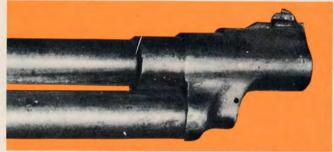
The massive muzzle piece on the Standard served as a housing for the bleeder valve and the gas cylinder, while hosting the blade front sight.
