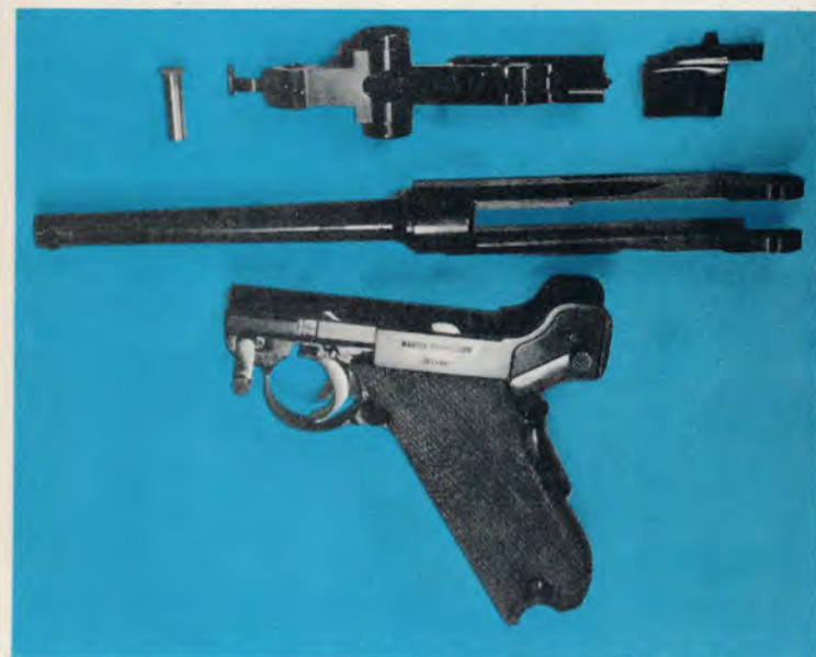
Field stripped, the Mauser Parabellum shows the very traditional parts. It is obvious that there have been no cost-cutting shortcuts used to produce this pistol.
