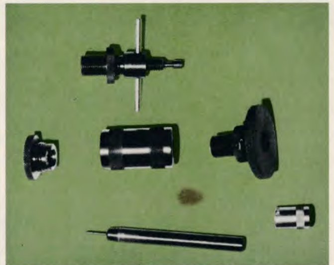
Pacific "Packit Tool." Clockwise the parts are: primer and bullet seating tool; neck sizing tool; charge cup; decapping rod; shell holder; and in center is die body.
