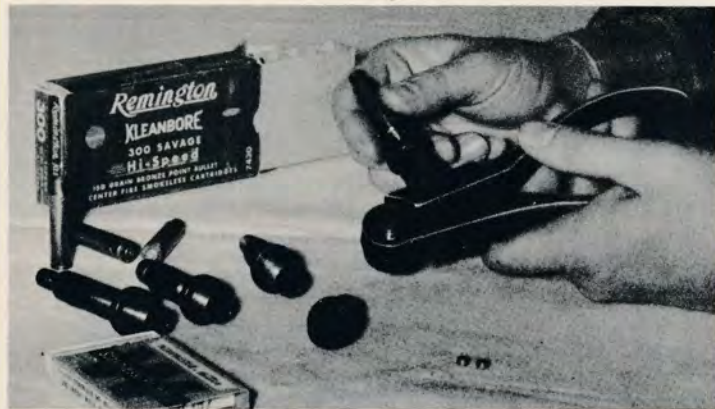
Lyman's "old reliable" No. 310 reloading tool is one known to many reloaders. This is an old tool with five dies instead of the present four-die set. Works well!
