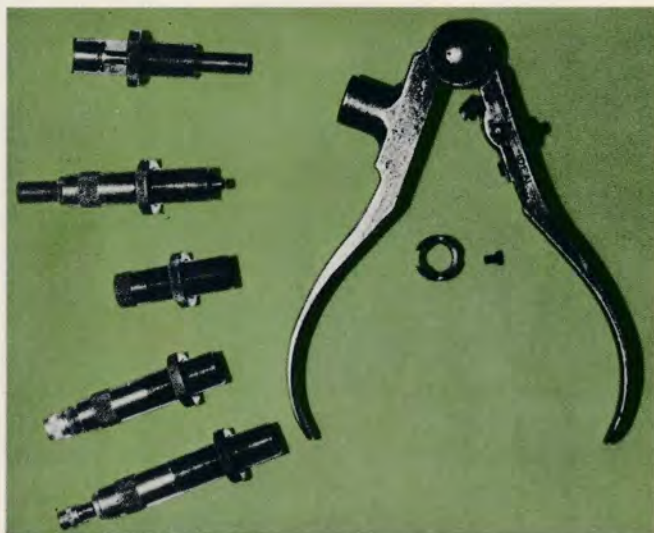
The Lyman Ideal #310 tool with the cartridge holder between the handles. Current sets combine decapping and muzzle resizing (neck sizing) in one die alone.
