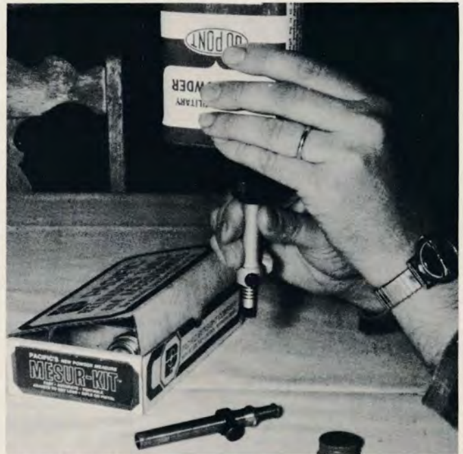
The Pacific "Measuring Kit" in operation. Extra charge tube is the Belding & Mull "Visible" measure. It is fully interchangeable with tube provided by Pacific.
