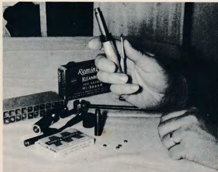
Lee's priming tool is available as an accessory for regular Lee Loaders or as a standard component for the Target Model loader. This is a very handy accessory.
