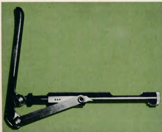
This side view of the W.H. English "Pak Tool" shows the linkage of the toggle system and the shell holder in place. This is the most expensive of the portables.
