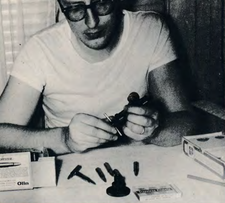
Pacific's new "Pakit Tool" uses silent screw-action for all operations. Here, the author is shown priming the case by the easy screw-in method that is noiseless.
