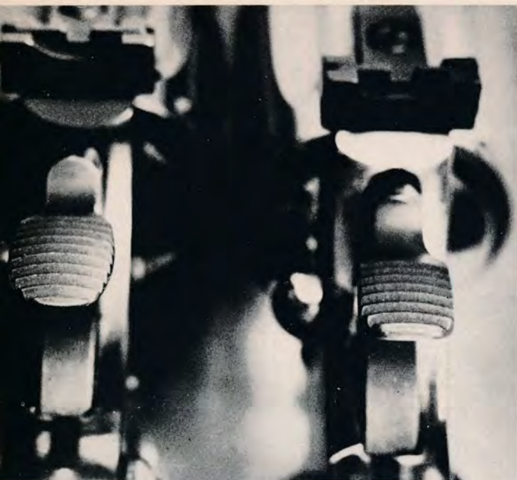
Regular hammer spur on the Diamondback (left) is much too wide and long, says Mason. The hammer on the right shows the bobbled length and trimmed sides as described in the text for better control.
