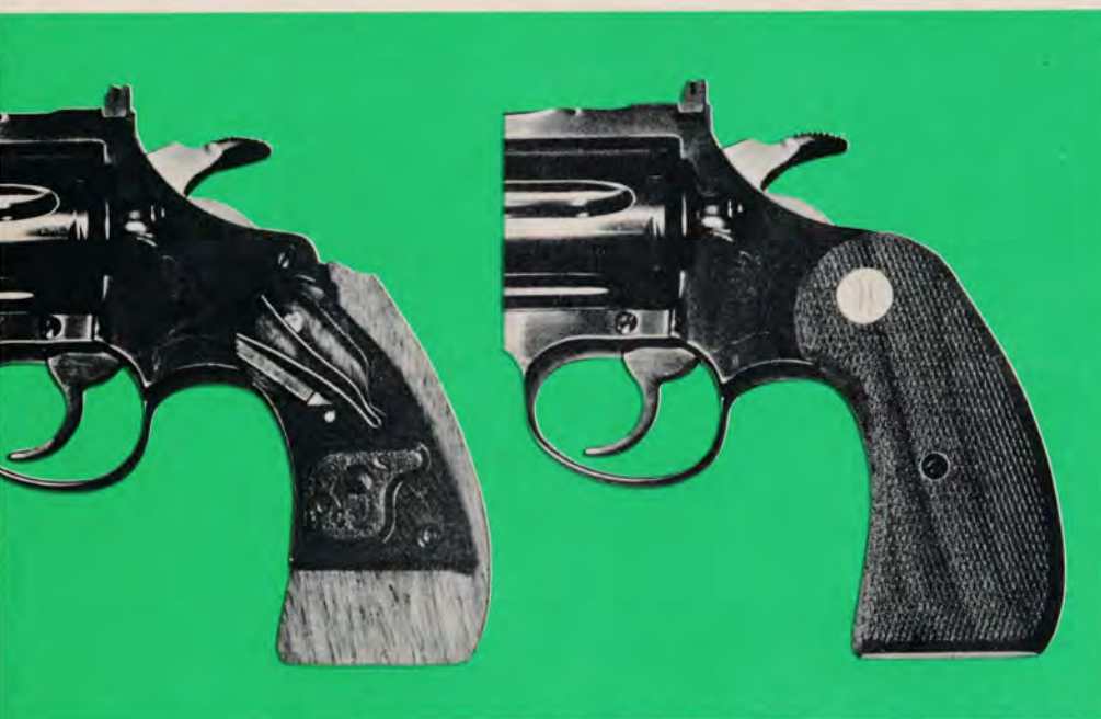
Herrett's service Shooting Ace stocks are concealable and aided point shooting compared to the standard factory stocks. Cut-away view shows the distribution of wood along the back strap that fills the hand and absorbs recoil energy. The generous field of checkering also aids in holding onto the gun during rapid fire strings. The general dimensions of the grips are adaptable to small-handed shooters and to the fair sex, making them quite popular. The Shooting Ace improved the author's point-shooting scores significantly with the Diamondback, compared to factory-supplied stocks.
