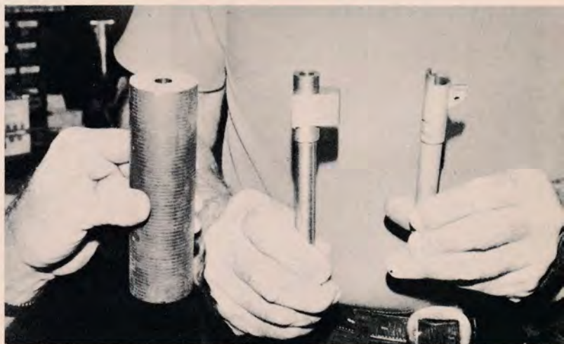
Barrels and slides in various stages of completion. Some have barrel positioners and sights installed.
