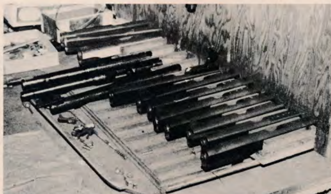
Barrels and slides in various stages of completion. Some have barrel positioners and sights installed.
