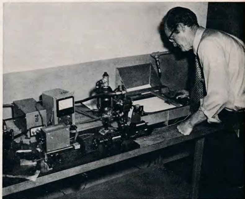
One of the many Winchester quality control tests is shown here with Thomas Sheridan at a trigger trace machine. Since the trigger/sear assembly could be considered the heart of a firearm, this machine may be called the electrocardiograph of the gun industry. The resultant graph is studied carefully by the experts.
