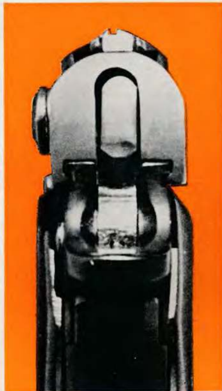
New-type combat sight used on the Asp is easy to use and is quite effective. No front sight is employed.
