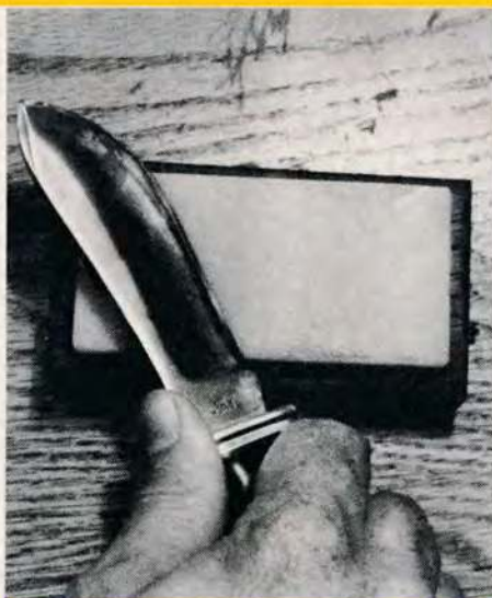
Left: This hunting knife is sharpened by moving the blade from left to right across the stone. Also the blade is pulled to the rear so that the point will be sharpened too. Right: Now do the same thing for the other side of the knife blade, drawing from right to left.
