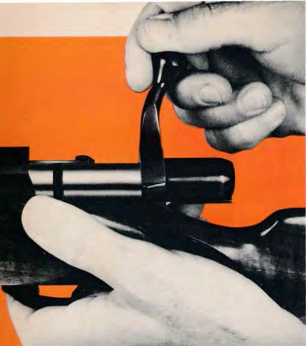
The bolt is removed with a conventional bolt release on the left side of receiver, which also contains the bolt stop and the ejector.
