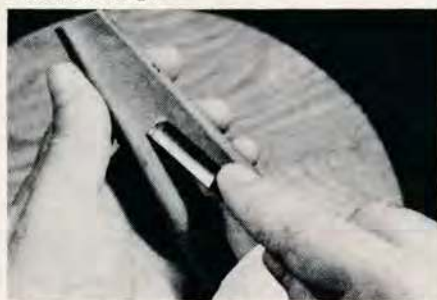
Sharpening outside edge of a gouge.
