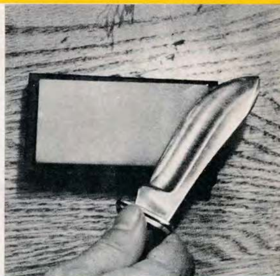
Left: This hunting knife is sharpened by moving the blade from left to right across the stone. Also the blade is pulled to the rear so that the point will be sharpened too. Right: Now do the same thing for the other side of the knife blade, drawing from right to left.
