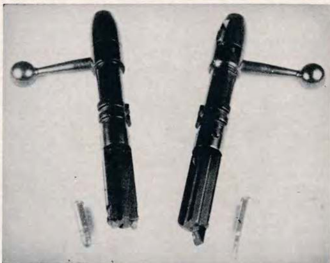
The series 580 bolt, left, has dual extractors for .22's while the 590 bolt (5mm) has a big hook.
