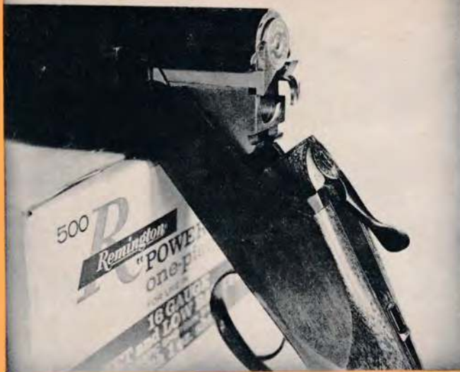
In this view, the lower barrel has ejected a case; top barrel has extracted unfired shell.
