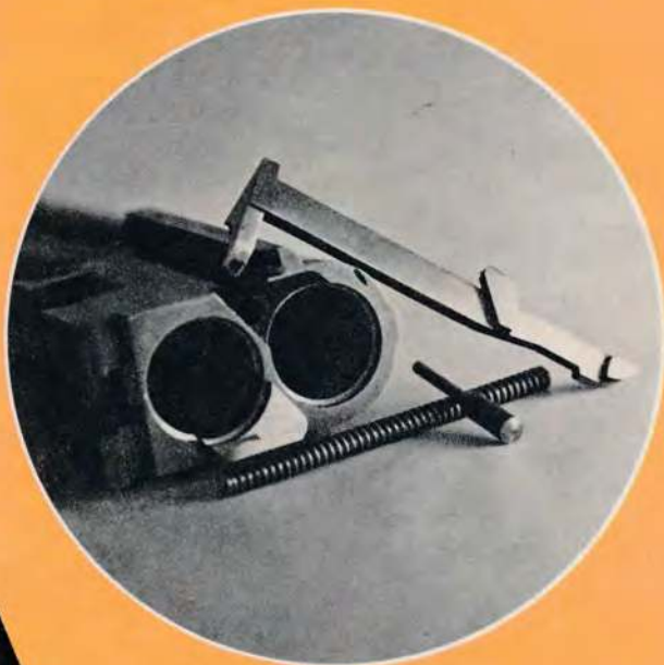
Monoblock breech houses major parts of the ejector system.
