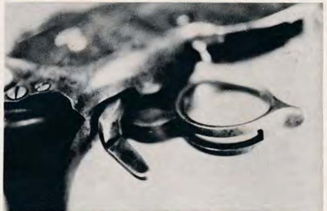
Close-up of the trigger guard lever ring. Slot at the rear of the ring is for the unusually shaped trigger.
