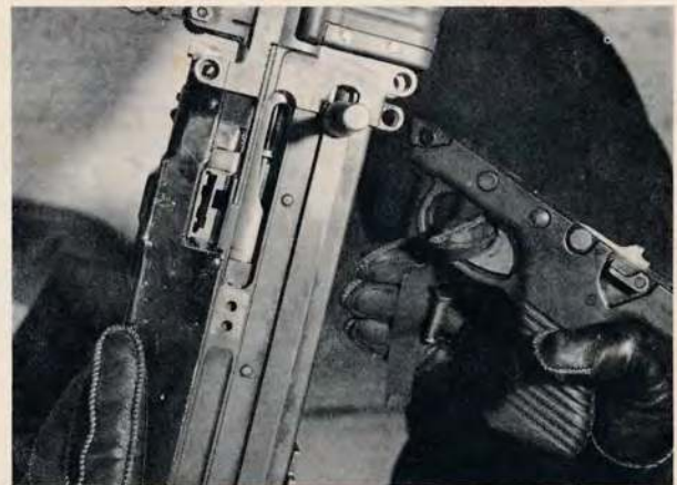
Above: The trigger group is easily removed from the receiver group by unspringing a flat spring and removing the cross pin shown. Below: Large lever near the carrying handle is merely pushed up for the quick removal of the barrel assembly.
