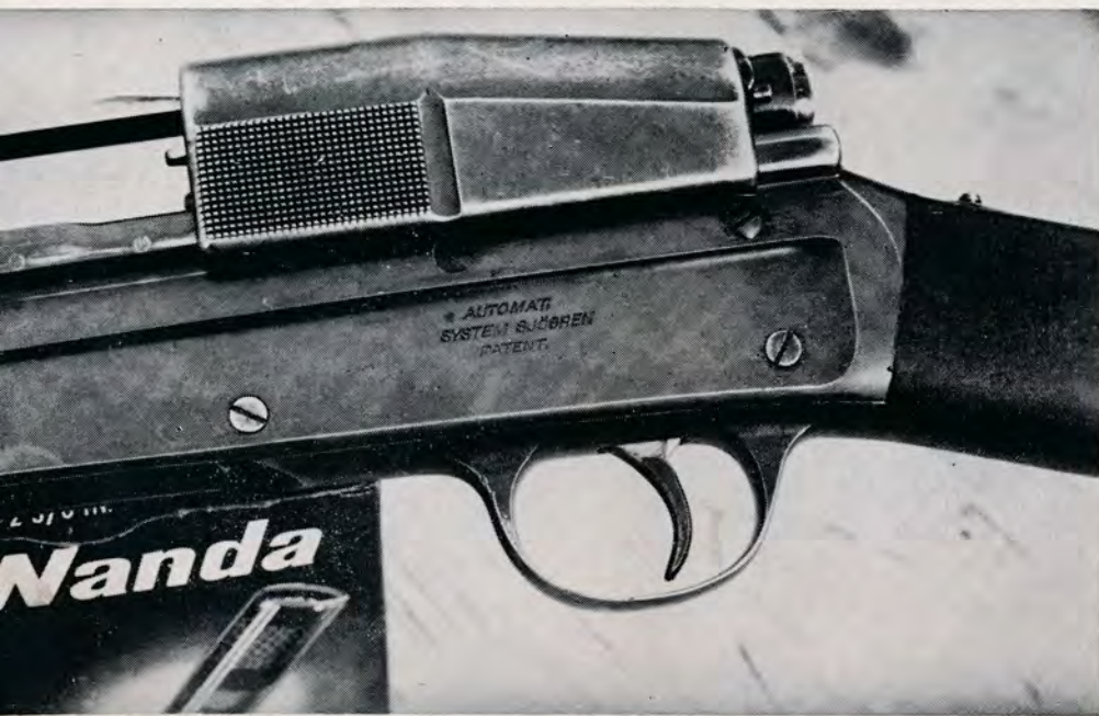
Left side view of the Sjogren showing the breech block in its full recoil position. Date of production is somewhere between 1903-1907.
