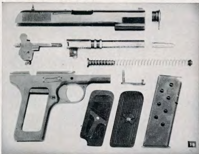
Tokarev field stripped. Note characteristic removable hammer group, the locking ridges around barrel, slide stop retaining clip on the right side of the receiver, and the metal "T" grip retainer on the inside of left grip.
