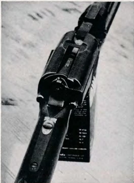
Sjogren has one Mauser-type safety to lock the firing pin, other is of the tang variety.
