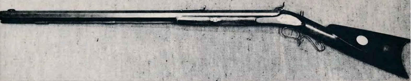
Above: Left side view of an Allen-Koppikus rifle. Note inlay in the cheekpiece. Below: Right side of rifle. Weight, 17 lbs., barrel length, 34 inches, .36 cal.
