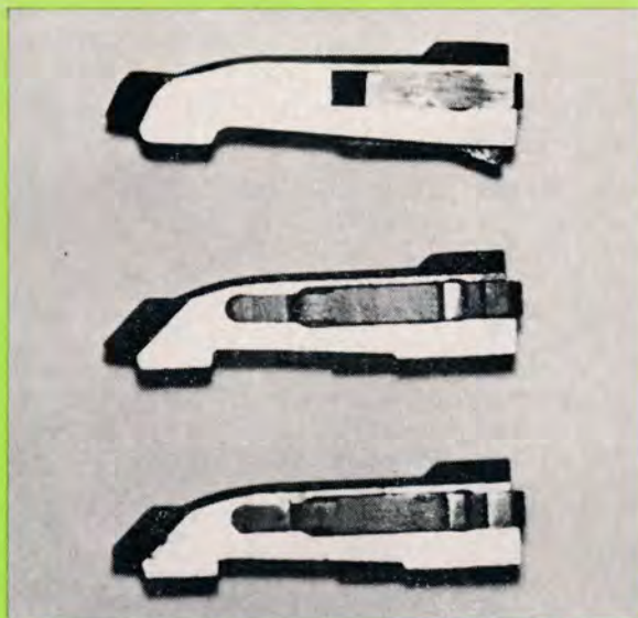
Three variants of M/51 breechlock, with a cam-operated (top) and early .380 (bottom).
