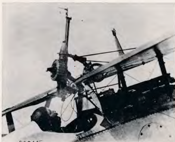
A .303 Lewis gun with a single fixed .303 Vickers mounted on a French Nieuport 27. Lewis was used as a back-up gun.
