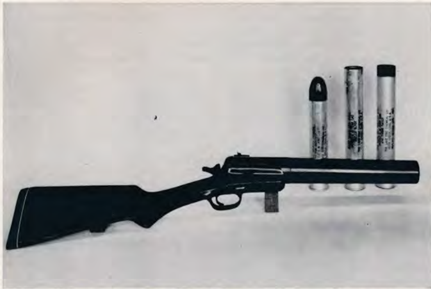
The conventional police 37 mm single shot tear gas gun. It weighs about 8 lbs., costs over $93, and fires short and long range tear gas rounds.
