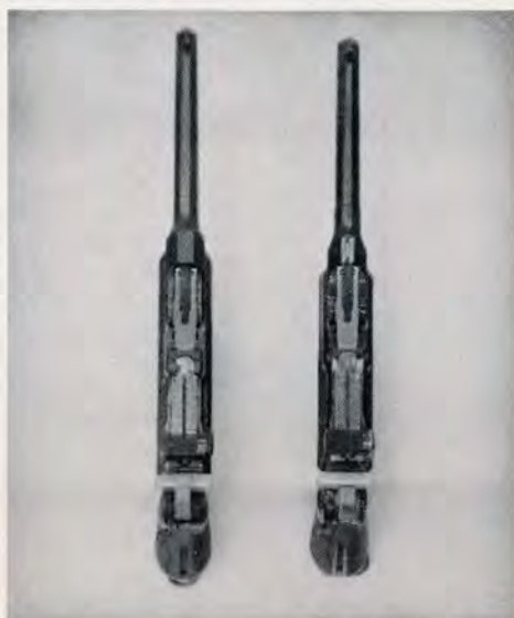
The barrel of the Mauser (right) is stepped, the sights are graduated differently and name is on chamber.
