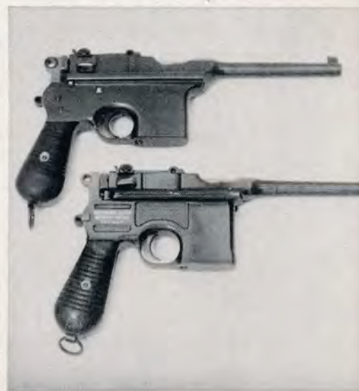
Action pins are evident in Astra. Overall finish is better because of different bluing process used.
