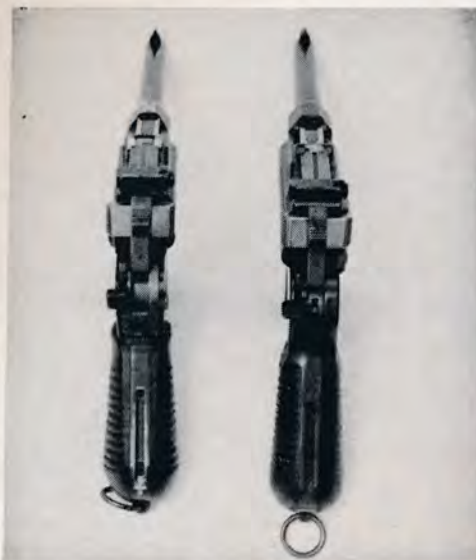
The Astra (right) shows differences in the hammer, barrel extension and the overall area of the back strap.
