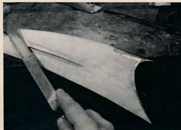
Fig. 7: Blending cheek-piece with rasp.
