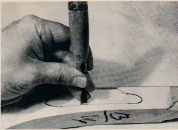
Fig. 4: Deepen outline with wood chisels.
