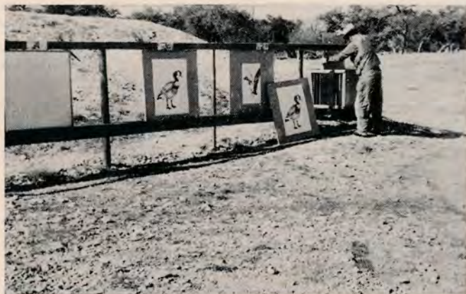
Running pattern tests at long range with the 10 gauge magnum. This testing also included penetration tests.
