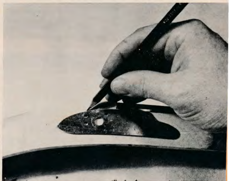
Fig. 3: Begin inletting the lock plate by tracing outline
