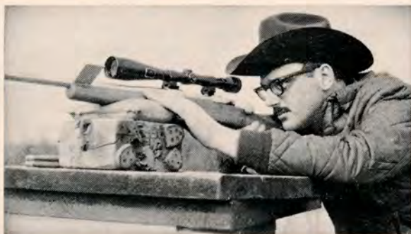
Author tries fore-end pressure test with thin paper shim exerting pressure against barrel.
