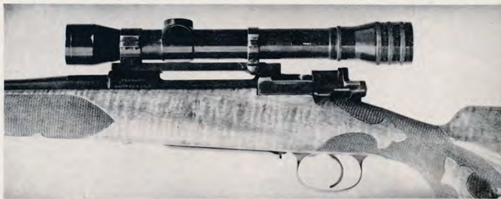
Top: Example of too much front overhang. Above: Example of too much rear overhang. Both ailments could have been solved by special scope mounts. In both cases the scopes were positioned correctly for right eye relief.
