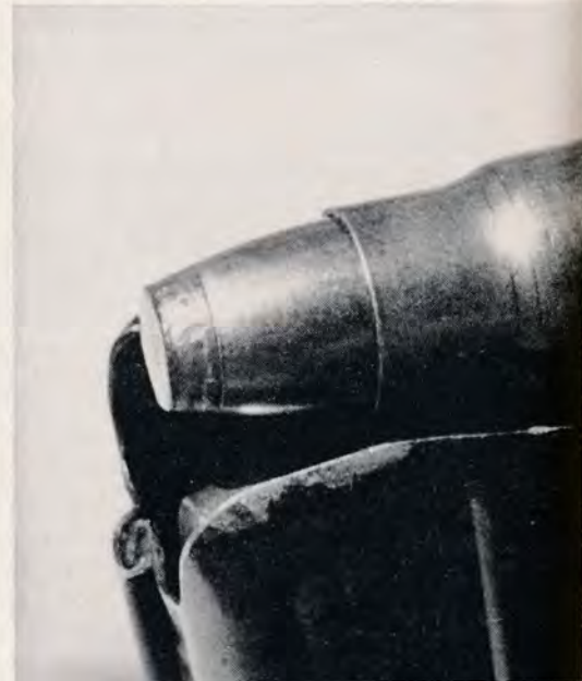
Fat Kurtz cartridges normally tend to find the center of the magazine. Lips of GI magazine must be pinched for case alignment with the breech.
