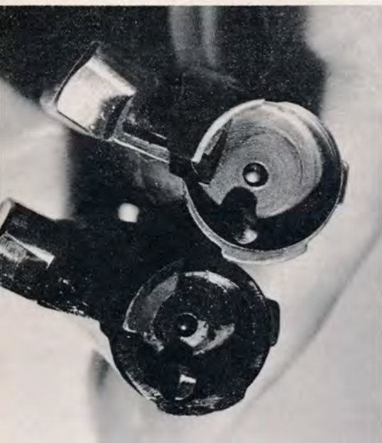
Extractor claw and bolt face must be machined to accept new shell.
