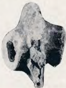
The two bullets, welded into a single mass, in a million-to-one chance. From the display at the U.S. Ordnance Museum at the Aberdeen Proving Ground, Aberdeen, Md.
