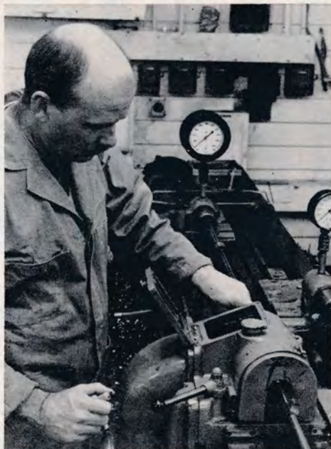
Bo Clerke of Clerke Technicorp inspects the set-up on a boring machine. Bore diameter being checked for consistency with air gauge for accuracy.
