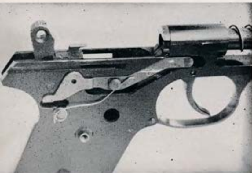
Above: TPH ejector is a simple stamping. Rounded nubbin serves as a disconnecter. Below: TPH fits well into a woman's hand.
