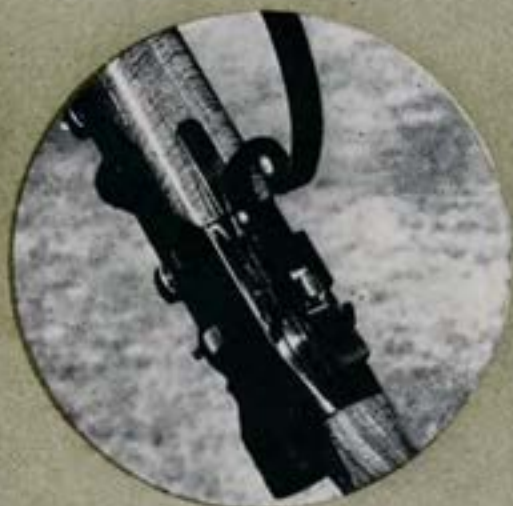
Top: The Sharps action open. The engine-turned breechblock plus the Timken needle bearings make the action a joy to operate. Bottom: The forestock is attached to the rifle by a hanger just ahead of the lever.
