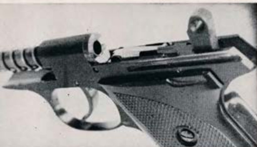
Above: Accuracy and reliability are easier to come by with the frame mounted barrel.
