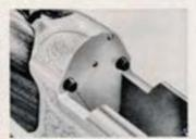
HARDENED STEEL BOLTS firmly lock the barrels to the receiver. MONOBLOC BREECH is stronger, since machining is done before barrels are inserted.
