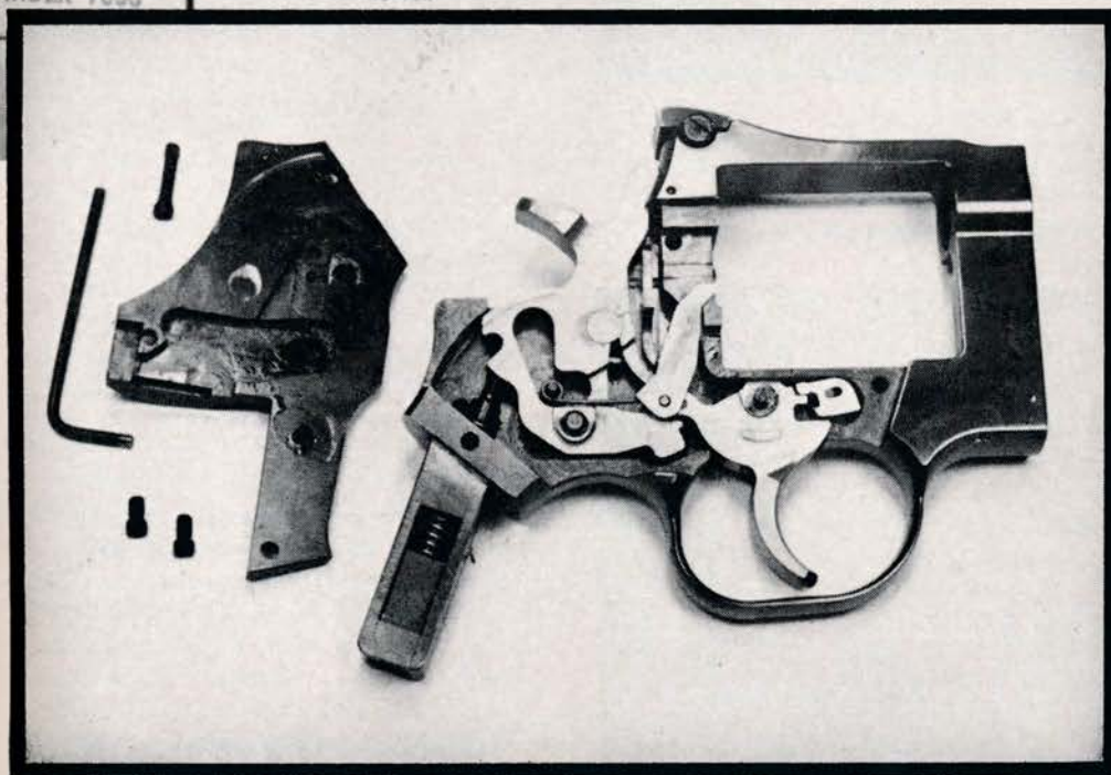
Above: the Dan Wesson Arms revolver, cal. .357 Magnum. Note the distinctive profile and muzzle. Photo of lockwork, left, shows the simplicity of design. Hammer spring is housed in the grip lug at rear of main frame.
