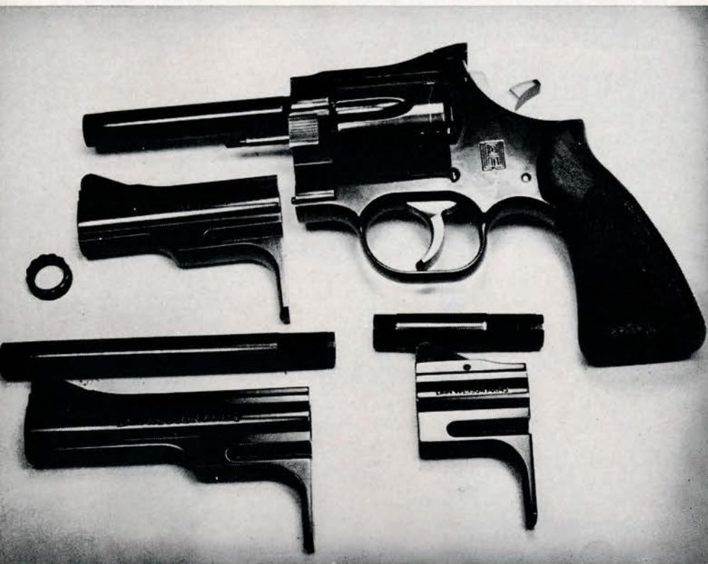
Above, the Dan Wesson revolver showing three barrel lengths with their respective barrel shrouds. Below, the grip slides up and onto the rear receiver lug and is secured by an allen head screw. Wrench is supplied with gun. Note the Dan Wesson trade mark on receiver.
