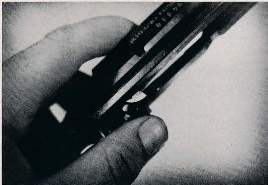
Top: Swedish L-40 locking system detail. Above: The locking block, with arrow which must point toward muzzle in reassembly. Below: Lahti's barrel group with the unique accelerator tail visible just above the thumbnail.
