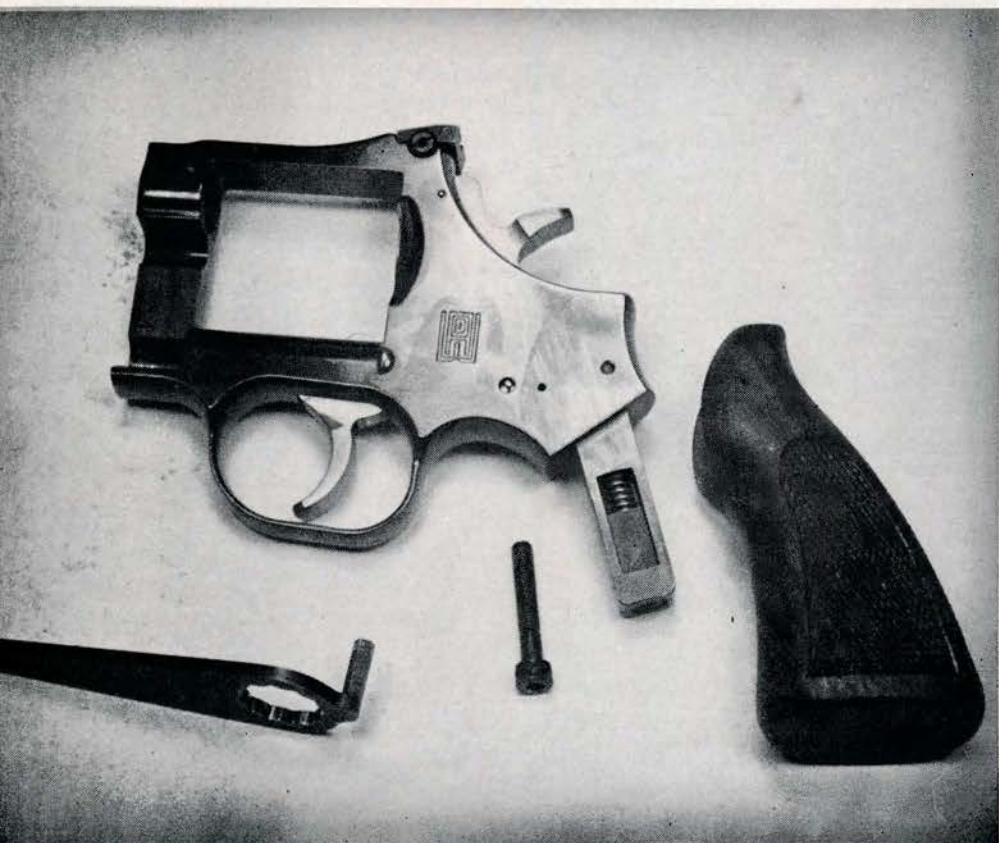
Above, the Dan Wesson revolver showing three barrel lengths with their respective barrel shrouds. Below, the grip slides up and onto the rear receiver lug and is secured by an allen head screw. Wrench is supplied with gun. Note the Dan Wesson trade mark on receiver.
