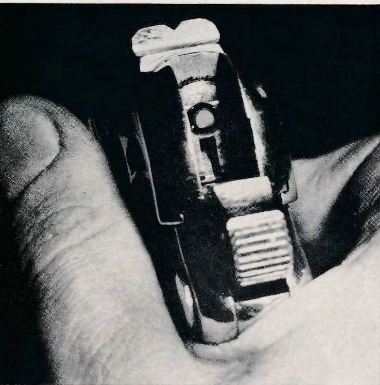
The rear of the firing pin can be seen extending from its tunnel in the breech block, before the safety is pressed.
