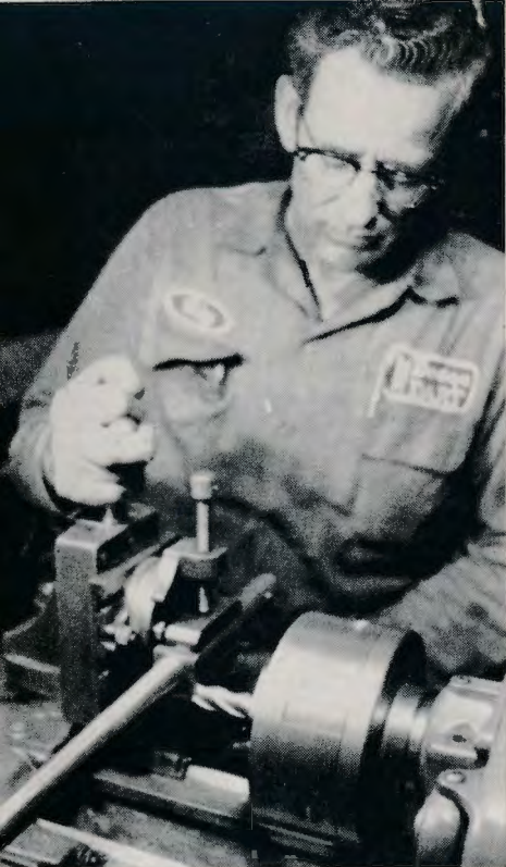
Here Clay Johnson mills a recoil lug. It takes about 25 hours to finish the actions on each rifle.
