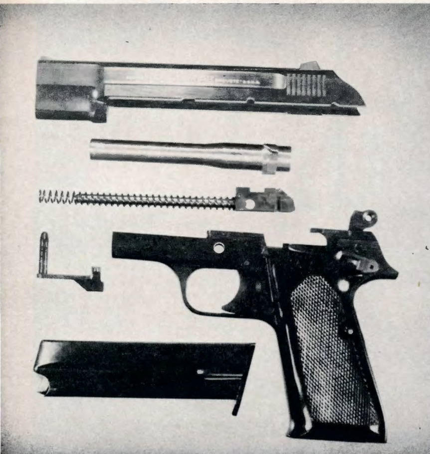
Field-stripped, the MAB PA-15 breaks down into six basic parts. (Note the simplicity of its components.) Compared to the Browning P-35 magazine (left) the MAB PA-15 holds an extra round.
