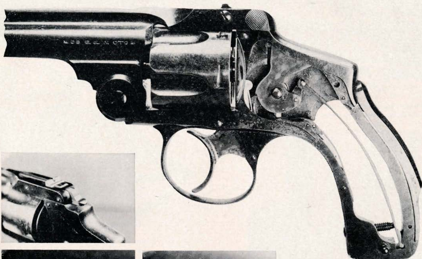
With sideplate removed, interior parts are visible. Photos at left show three of the variations used in the hammerless locking system.
