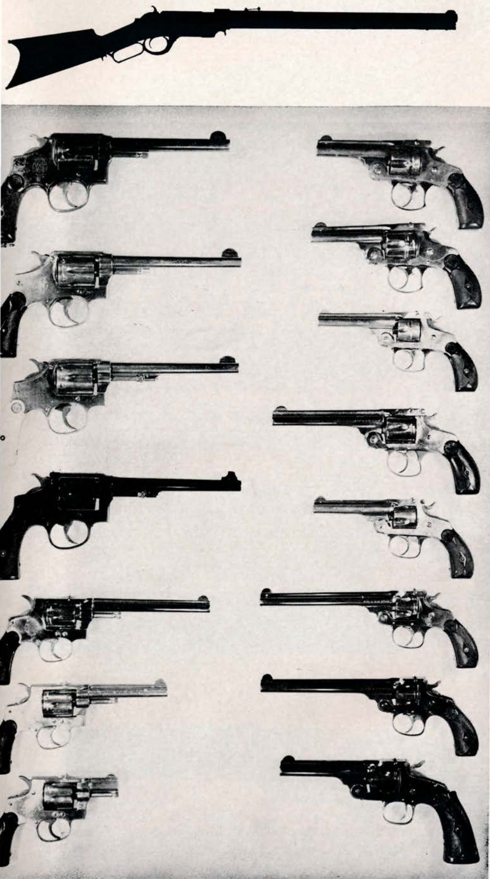
Under Daniel Wesson's direction, the top-break revolvers (right) were phased out and replaced by the improved models with the swing-out cylinders (left).
