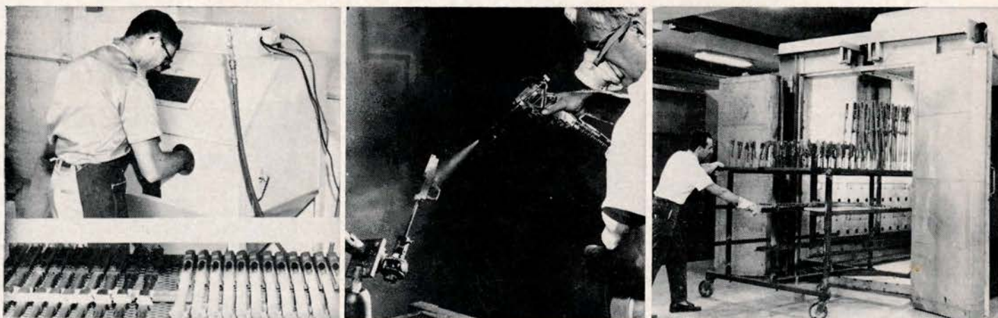
Steps in Teflon-coating process: sandblasting; spraying; baking.
