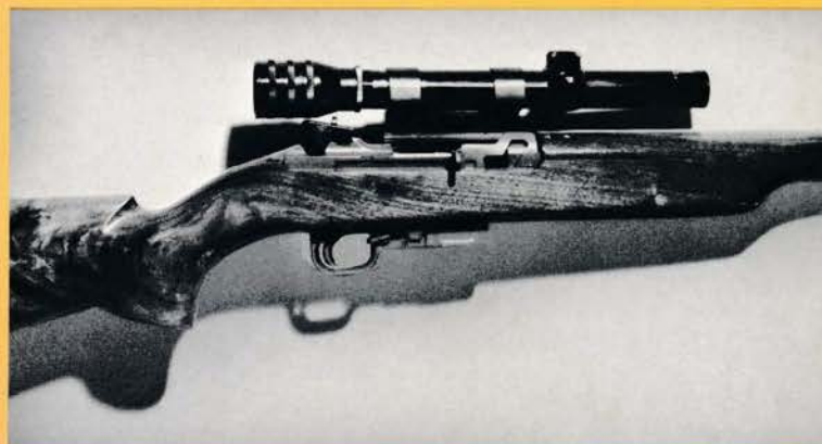
Test rifle, with Universal Model UD 4x20 scope mounted, looks like new after firing 500 rounds.
