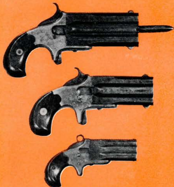
Wesson made several derringer models with rotating barrels, from .22 - .41 cal. r.f.; some were fitted with sliding knife blade. Top: .44 cal. carbine of Civil War vintage.
