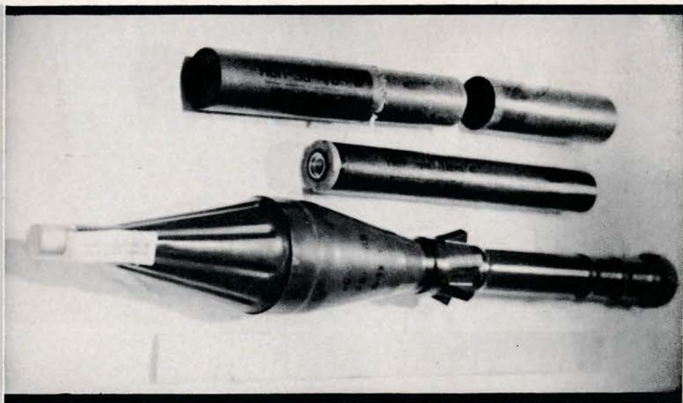
Left: The RPG-7 weighs 15 lbs, and has a range of 285 meters. Above: The RPG-7 rocket, broken down into components which are easily carried in jungle.
