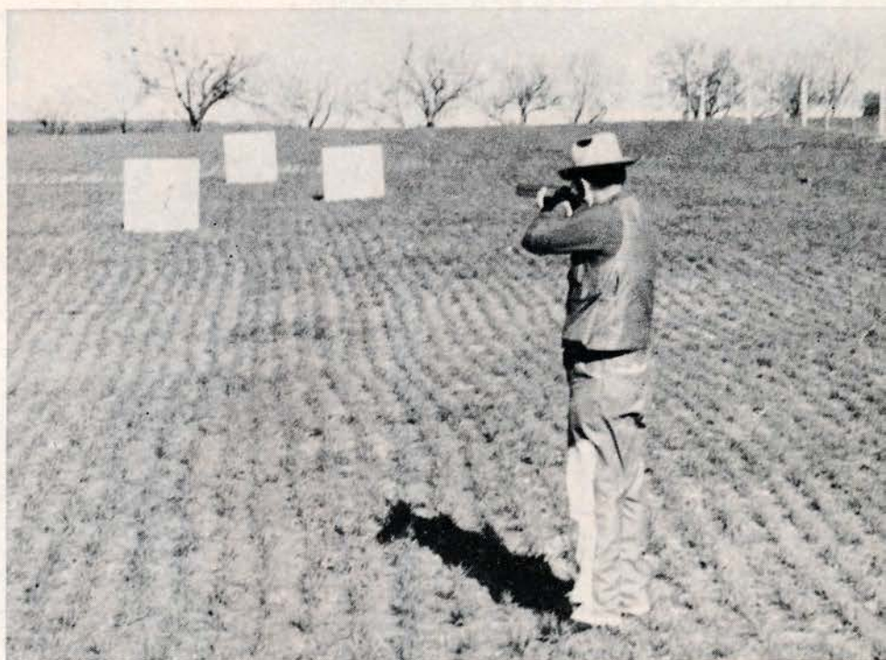
Askins pattern-tested the Lames at 25, 30 and 40 yds. and in all instances it indicated good distribution.
