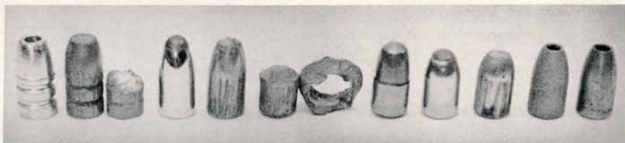
Before and after shots of various bullets fired into sand at 65 yards.
