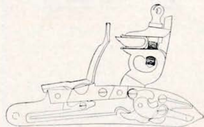
French carbine lock, circa 1815, had both flashpan cover bridle and tumbler bridle, improving function and timing.
