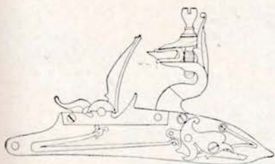
Good quality lock of 1780-1825 used a better, friction-reducing linkage, had curved shield to protect pan from rain.
