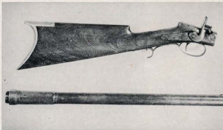
A caplock "goose gun," patented by Wesson in 1847, has screw barrel with seven bores producing lethal pattern.
