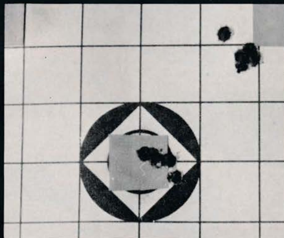
Left: Cutaway cases show that most commercial ammo is loaded with bullets seated into case. Below: Five shot groups, measuring about \frac{5}{8} " shot from a 6.5 caliber Remington 660 carbine.
