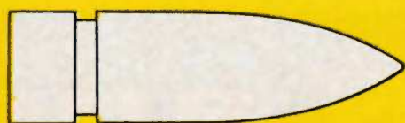
SQUARE SHOULDERED CANNELURE WITH SMOOTH FINISH
