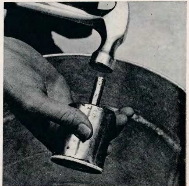
The tincan die holds shell for foolproof hydraulic depriming. Below, the Poorman's Primer Pusher does a quick job on the big obsolete militaries.
