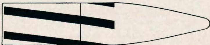
Flat base bullet fired from a barrel with right hand twist.
