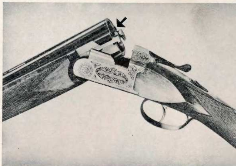
Beretta has developed a system using lugs on the barrel breech which lock into recesses in the standing breech.
