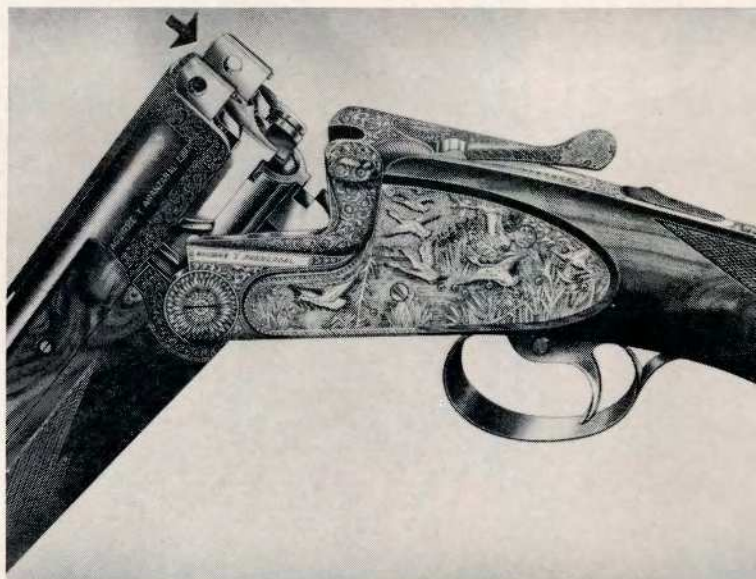
The Spanish AYA has a Merkel-type action which uses two Kersten fasteners positioned alongside the top barrel.
