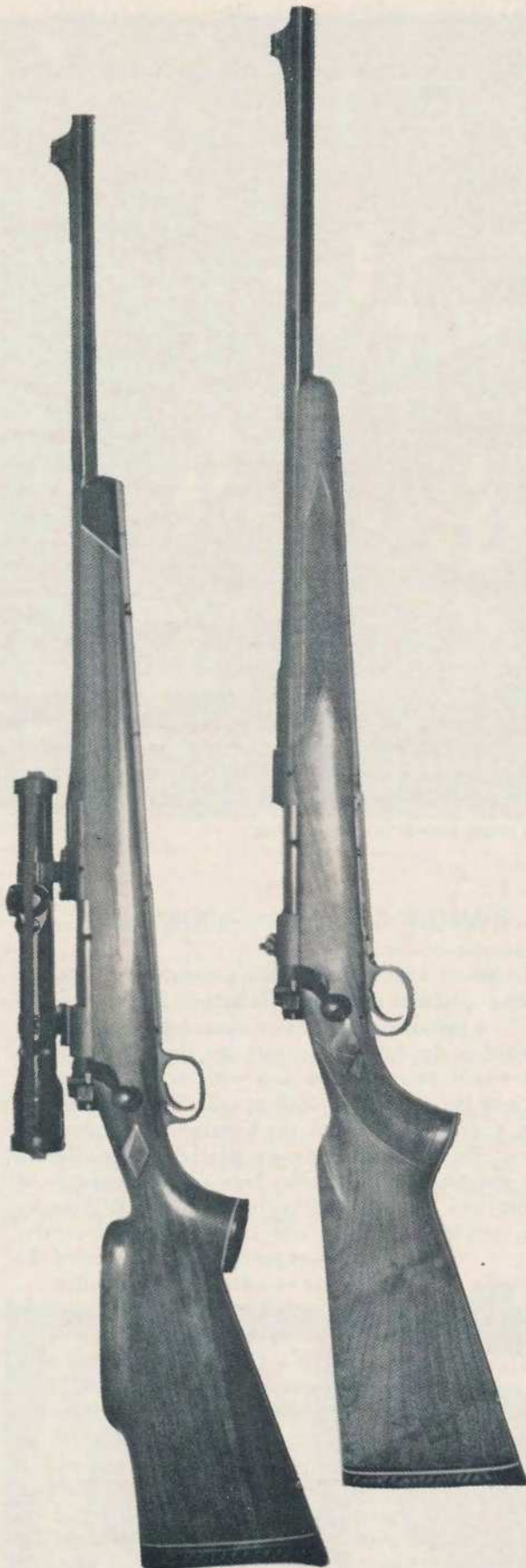
In 7 mm Magnum and .333 Magnum wildcat, these Model 70's have interchangeable bolts.
