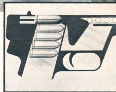
Schematic cross section of rocket handgun shows how rockets are stacked in magazine. Left, cocked and ready to fire; right, hammer drives rocket into firing pin. As rocket starts down barrel, it re-cocks the hammer.
