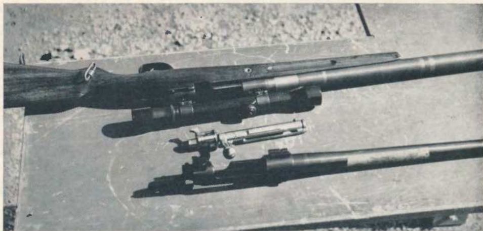
Military stock, trigger, bolt, and scope were switched back and forth between heavy barrel and light sporter barrel. HB gun weighed 15 pounds with scope, and recoil was less than that of '06, sporter recoil was equal to '06 kick.
