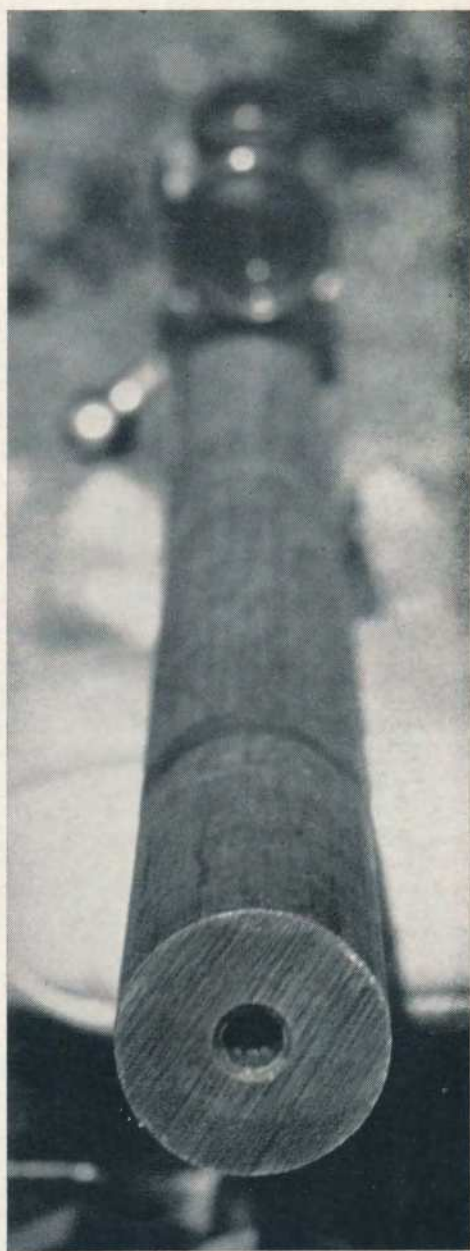
Military stock, trigger, bolt, and scope were switched back and forth between heavy barrel and light sporter barrel. HB gun weighed 15 pounds with scope, and recoil was less than that of '06, sporter recoil was equal to '06 kick.
