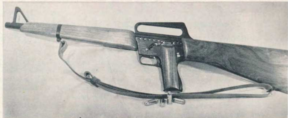
The rocket carbine is shown here without turbulence deflector which adds 1½" to 34" length. Standard 13 mm rockets are shown with the test carbine.
