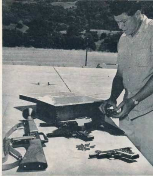
Mainhardt loads rocket guns; note .45 ACP gun, ammo. Near barrel is that of production gun with steel liner; early channeled, unlined barrel right.
