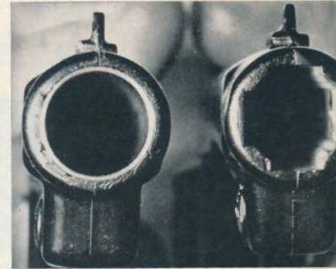
Mainhardt loads rocket guns; note .45 ACP gun, ammo. Near barrel is that of production gun with steel liner; early channeled, unlined barrel right.
