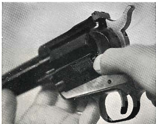
View above of Hawkeye shows breech block plunger in the closed and locked position.
