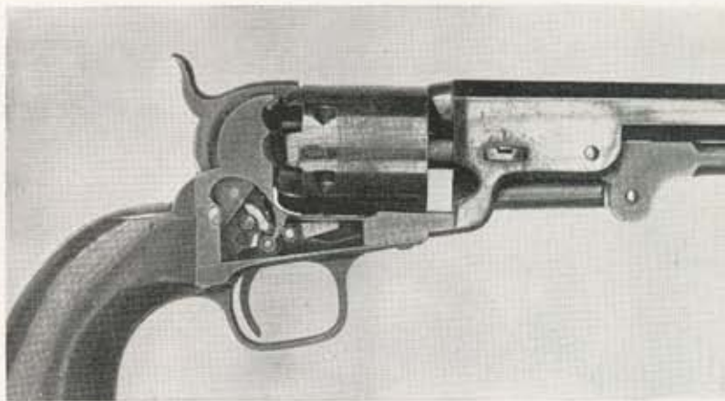
Most SA lockwork designs are development from old Colt Navy 1851 system (above, shop model). Cylinder bolt rocks off hammer stud to disengage as gun is cocked.
