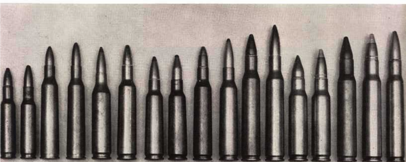
Though same in weight, 110 grain .30 and .270 bullets (above) show markedly different shapes.
