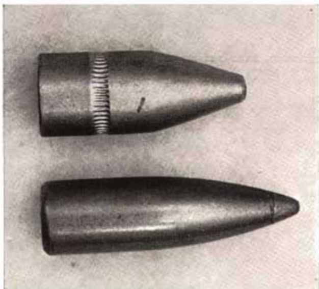
Though same in weight, 110 grain .30 and .270 bullets (above) show markedly different shapes.
