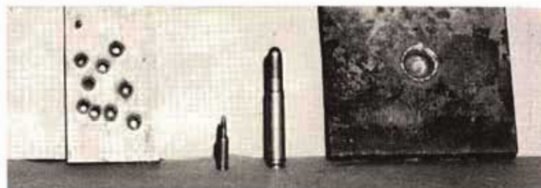
Plate at left shows how 17 Javelina cut through \frac{3}{8} " of steel at 50 yards. Cratered hole in \frac{3}{4} " steel plate at right was made by .475 Magnum. Note cartridge comparison.
