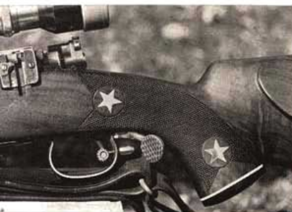
Built for fingerless firing is '98 Mauser with stud trigger. At right, M40 WRaco shotgun has slide hook; .22 has forearm knob.
