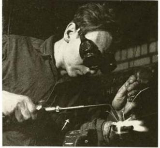
Water-soaked rags protect locking lugs, and goggles protect workman's eyes, as student welds bolt handle.
