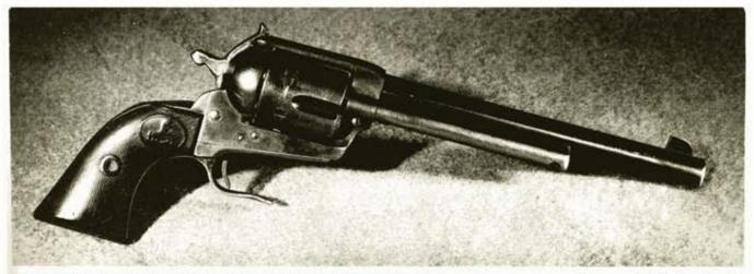
Colt Peacemaker was modified by western gunfighter for speed. Hammer spur was lowered to permit slip shooting by letting hammer slip from under thumb while cut guard allowed finger to hold trigger back, leaving hammer free to fall.
