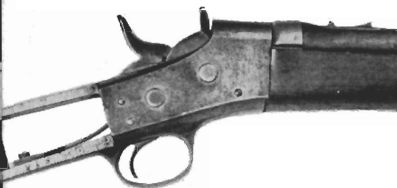
Remington receiver tangs must be bent and spring altered for large-size custom grips to take up kick.
