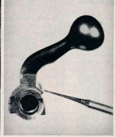
The large reserve safety lug directly beneath the bolt handle is a problem. It is reduced by about 60% as part of the conversion.
