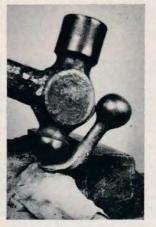
In the beginning blows must be at right angles to the bolt shank. Blows with ball of hammer are directed progressively toward body.
