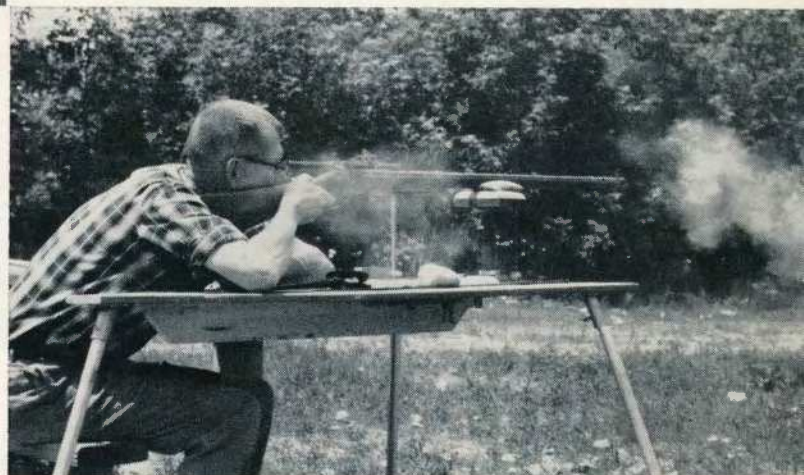
The newly converted muzzle loader produced a five-shot group that measured four inches. Not a bad first try.
