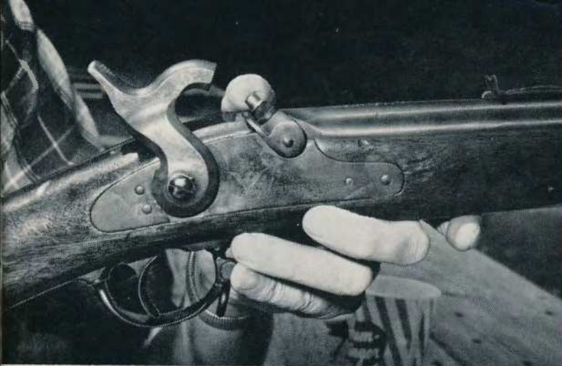
Fitting of the muzzle-loading barrel and hammer to the Springfield was quite easily and quickly accomplished.
