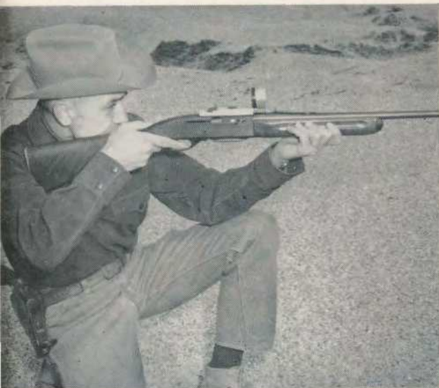
Using the Nydar's experimental polarizing attachment, the author found that it kept the reticle from fading in spite of the extremely bright sunlight and background.
