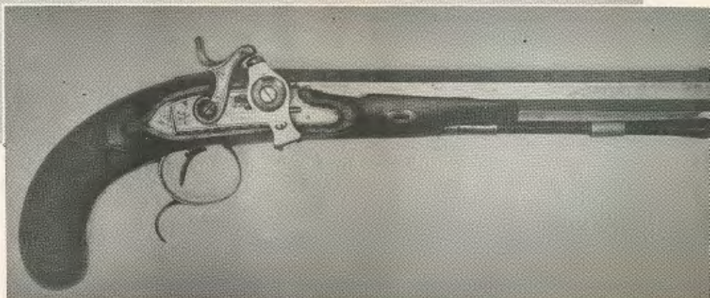
Right: Duelling pistol with a Forsyth lock. Note adjusting screws on each side of primer.
