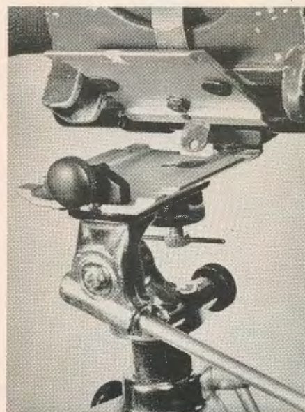
Author's spotting scope with its special tripod and the added aiming scope. Right: Close-up of the home-made detachable head.
