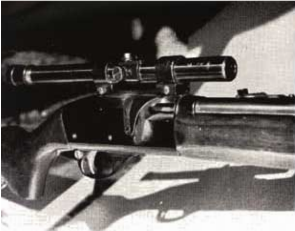
Shell shield on Rem .552 keeps hot brass from face, may kick them back into gun.
