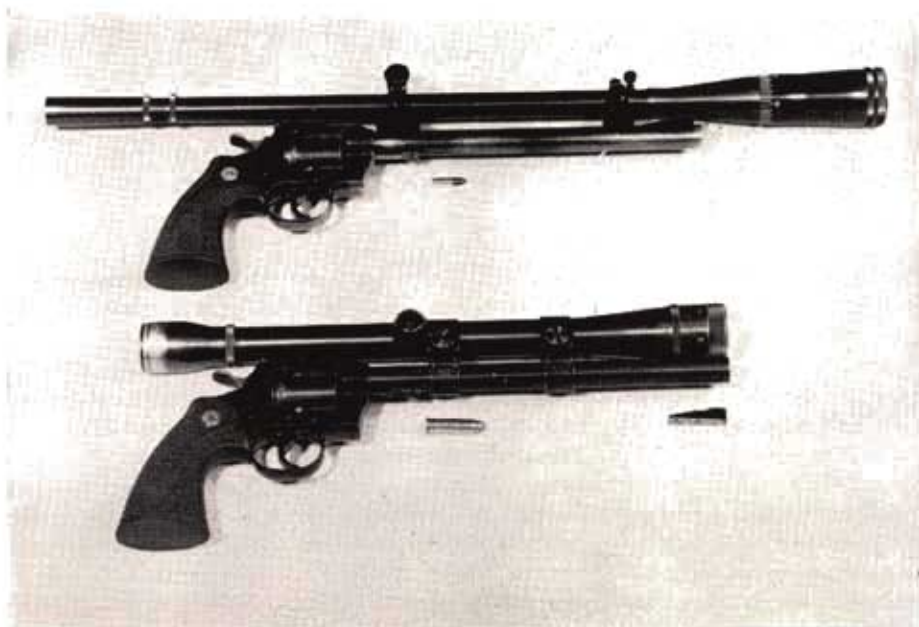
Officers Models in .22 (top) and .357 were fitted with special 10" barrels at Colt factory. Heavy .357 has Weaver K-10 in split mounts.
