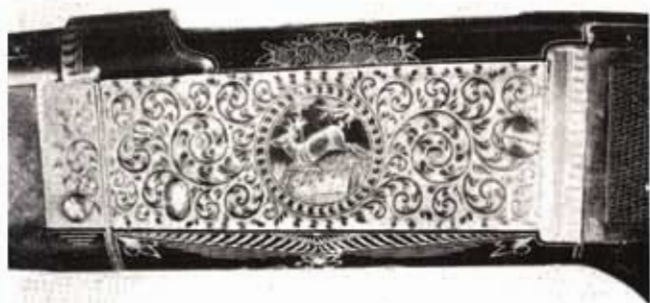
Flat-sided Savage receiver takes engraving well. M99K had ornate scroll pattern with game scene in vignette.
