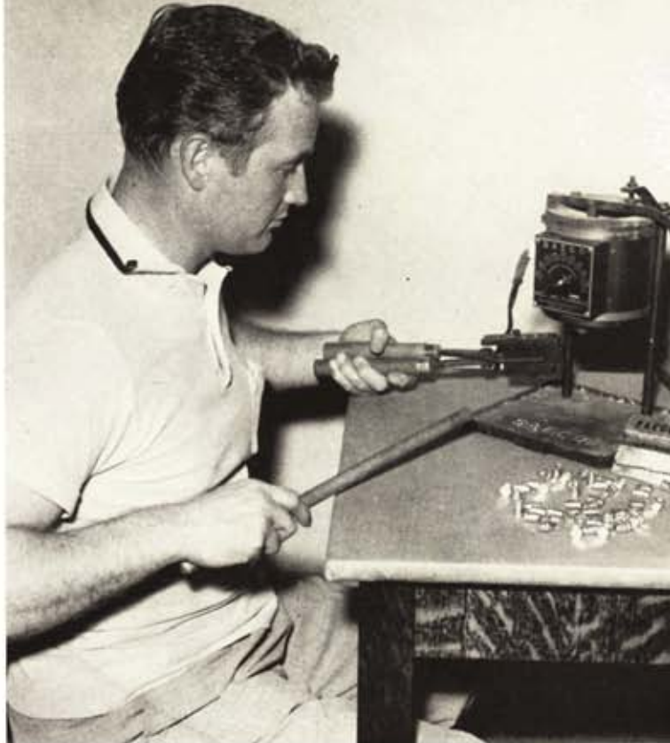
Handloader uses SAECO furnace to keep lead at constant temperature for best casting in Hensley-Gibbs gang mold.
