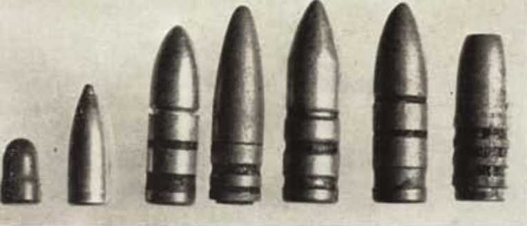
Tiny 4mm shell (left) is gallery load for insert barrels. Sisk Lovell 50 gr. .22 is good small game slug. Bigger lead bullets are Lyman 123 gr. .270 #280473; Harvey 135 gr. 7mm; Lyman 194, 169 gr. .30's; and Hensley-Gibbs 150 gr. .30.
