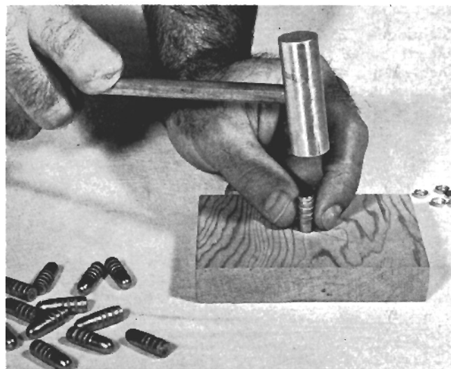
Hole in block holds tip as gas-check is put on base.
