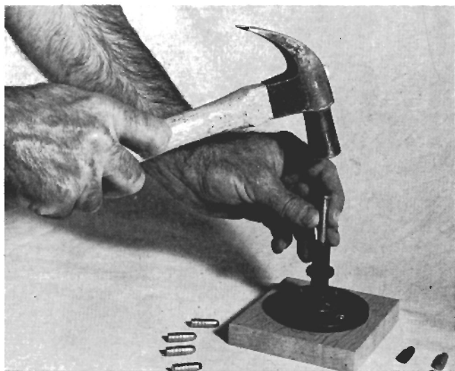
Bullets are sized through Ideal die in cheap pipe base.
