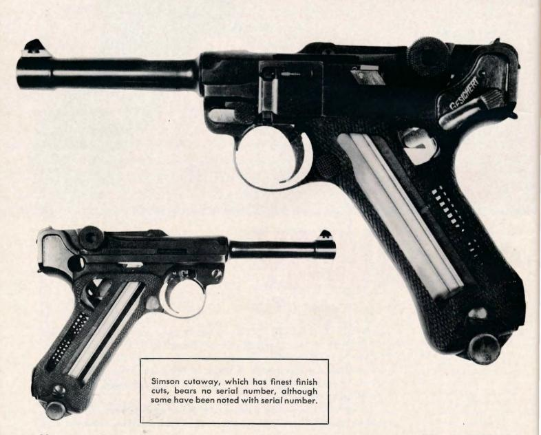
manufacturer's name, and is the only cutaway with a removable barrel. While the Mauser and Simson cutaways do not show their respective producers' names, the manufacturer can be determined by the proofs.
