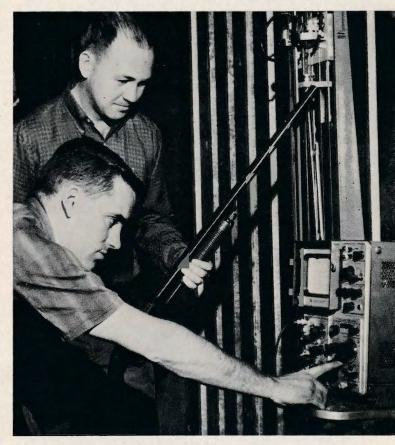
Bill Cranney adjusts oscilloscope prior to tests as Clair Rees looks on. (Note grid where recoil is charted as time vs. force curve; grid trace is photographed.
