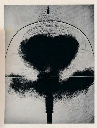
Right: Buckshot and wadding are frozen in midflight in this shadowgraph. Shock waves can be seen ahead of pellets; air turbulence is seen behind. Photo from U.S. Army Ballistic Research Laboratories, at Aberdeen Proving Ground, Md.
