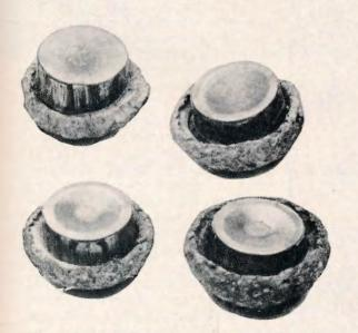
The .38 cal. bullets above and the .45 ACP bullets, right, show the type of expansion that provides good target stopping energy.
