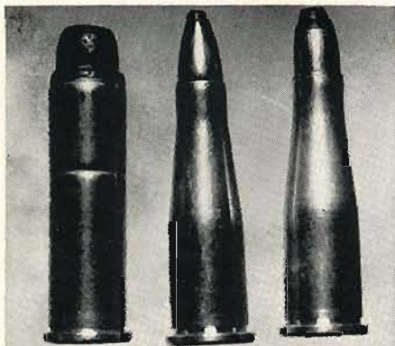
The .44 Magnum, factory-loaded .22 Jet, and Sisk-Bellah pill in new Jet case.
