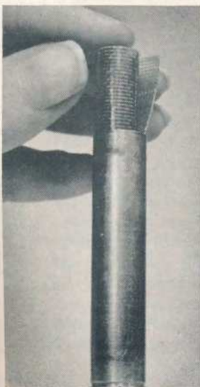
Left: Sleeve is rolled 2½ turns opposite the rifling twist. Right: Over-shot wad installed.
