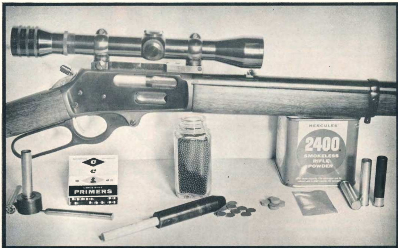
Items needed for shot-loading the .444, left to right: punch and base set; primers; wad cutter and ram; shot; material for the shot sleeve, empty cases, and powder. With these, the Marlin becomes a close range shotgun.
