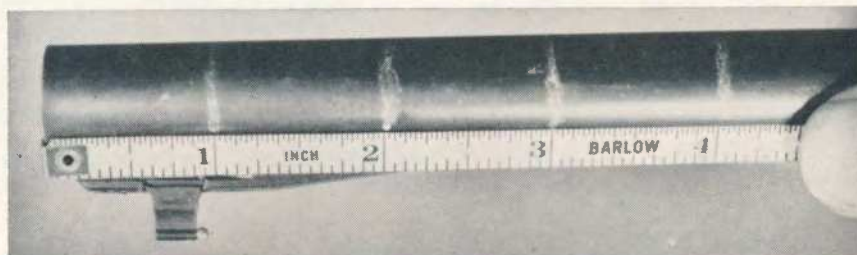
Removal of four inches of barrel from Marlin .444 scarcely changed the velocity readings, although muzzle blast was slightly increased.
