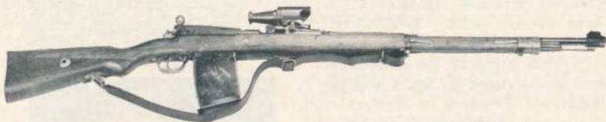
Mauser Gew.98 with special Zeiss "bifocal" sight.
