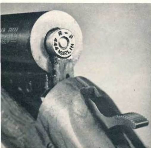
Left: Some .410 shotguns will chamber the .444 Marlin case, and this is dangerous. Right: The .444 case compared to .410 shells.
