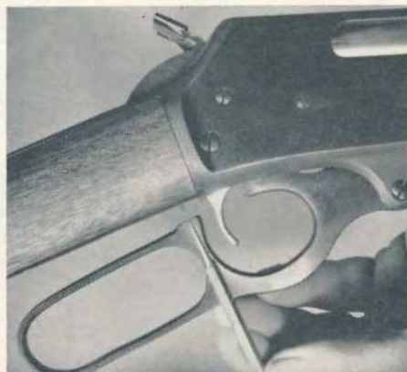
Left: The .444 has added grip safety. Right: Cartridge carrier has a spring loaded gadget (bottom) to aid feeding; 336 carrier shown above.
