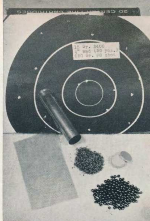
Small piece of glass sheeting (left foreground) which protected the shot, was key to shotshell's performance.
