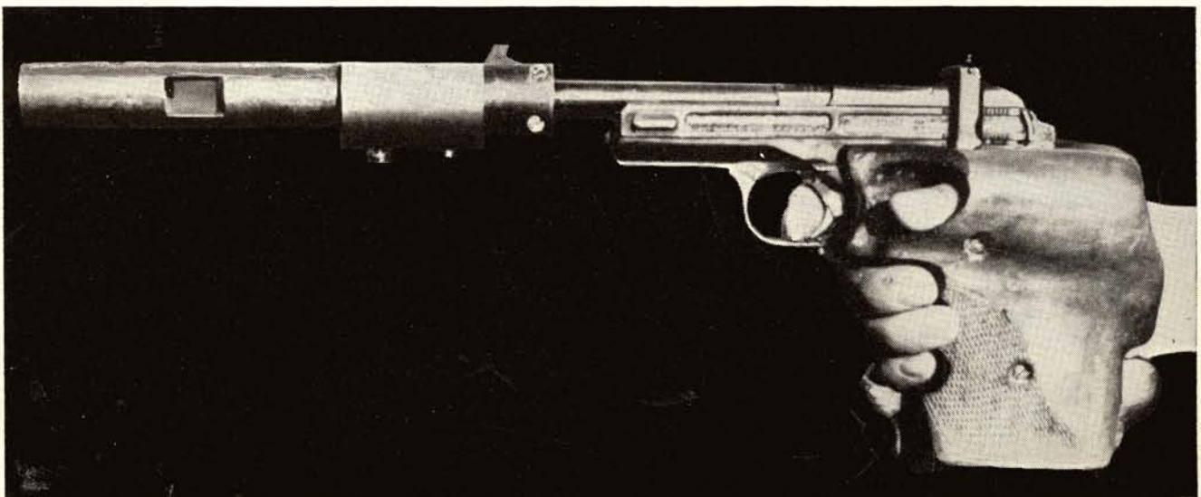
Rapid fire pistol used by Soviet pistolmen at Caracas was best of blind inventor's standard designs, had elaborate muzzle brake and weight with fixed rear sight bridge.
