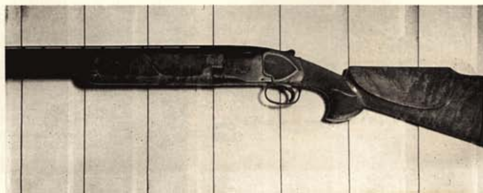
Main difference between trap guns and skeet or upland smoothbores is in choke constriction, but Grand guns evidence butt lengthening, special stocks and comb. "Etchen" pistol grip is liked by many experienced trap shooters.
