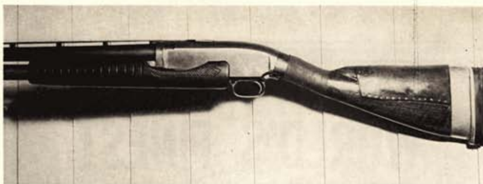
Much-lengthened Model 12 with built-up adjustable buttplate and extension forearm was worked over to give hopeful owner better chance of winning.
