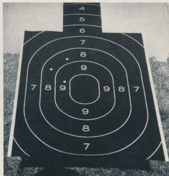
This .38 Special cartridge has three bullets which separate once out of the barrel giving close patterns at 20 meters.
